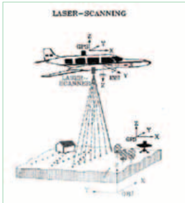
Figure 4.2.2.B/2.3 Diagram of laser scanner technology. Figur 4.2.2.B/2.3 Funktionsschema der Technologie Laser Scanner. Figura 4.2.2.B/2.3 Schema di funzionamento della tecnologia laser scanner.
