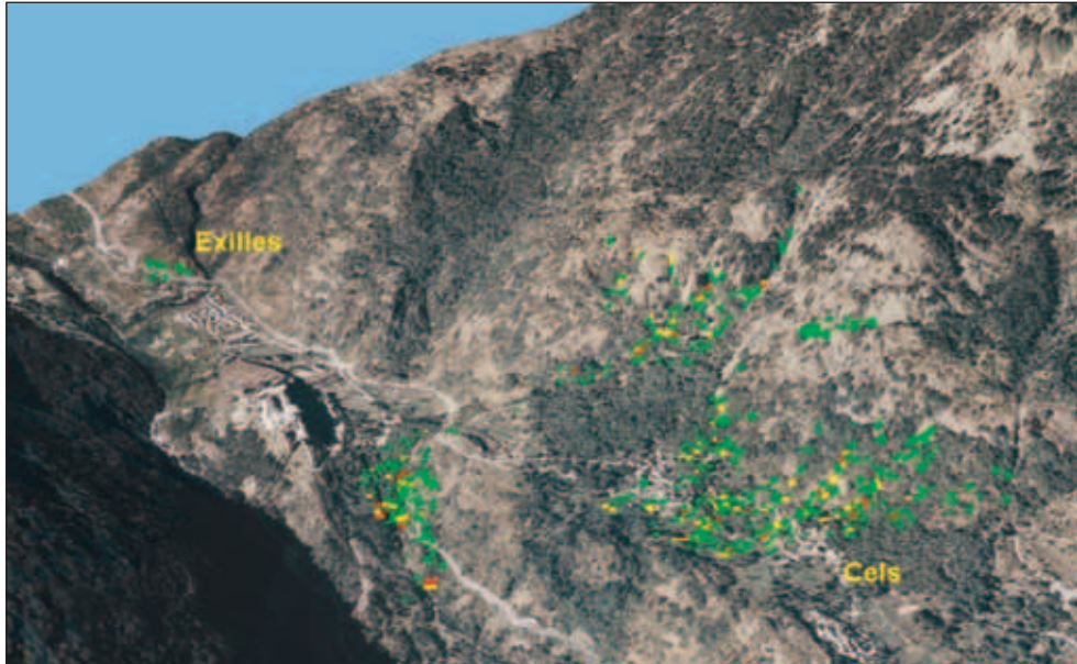
Figure 3.2.3/2.1 Distribution of stopping points of boulders after the rock fall simulation (the yellow and red areas show where most boulders stopped). Area of study: Commune of Exilles, left side of Val Susa, province of Turin.
